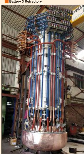
24 MVA Furnace Electrode Assembly
